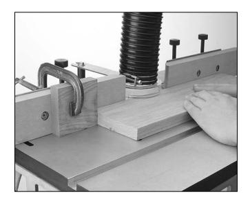
Figure 28. Stop block in position.
